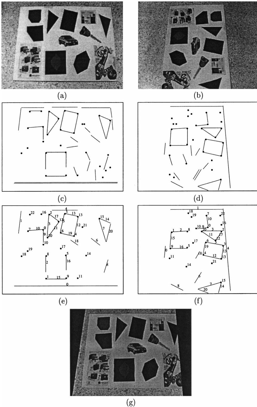
Fig. 3. (a) and (b) Two views of a poster. (c) and (d) The extracted features. (e) and (f) The computed correspondences. (g) Second view warped according to the estimated homography (see text for explanation).
