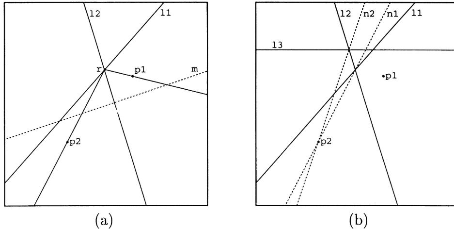
Fig. 1. (a) The pencil centered at  $r$ , defined by lines  $l_1$  and  $l_2$  and points  $p_1$  and  $p_2$ . For any line  $m$  intersecting the pencil, the cross-ratio of the pencil is equal to the cross-ratio defined on  $m$  by its four points of intersection with the lines of the pencil. (b) The dashed lines, defined by two  $2\mathcal{L}2\mathcal{P}$  invariants, intersect at  $p_2$  (see text for explanation).
