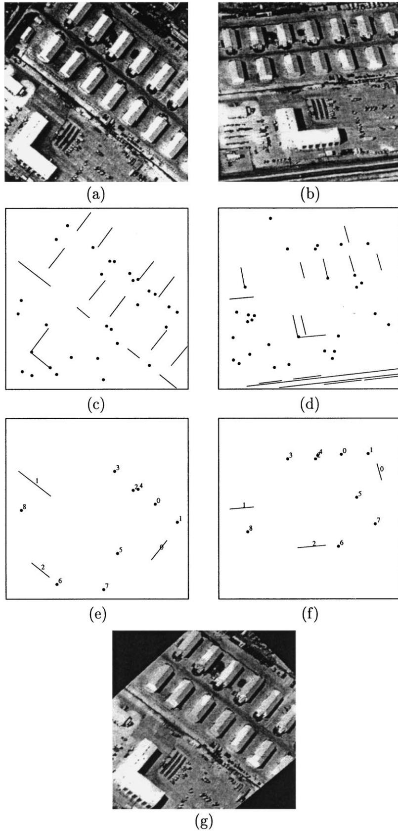
Fig. 4. (a) and (b) Two aerial images (courtesy of P. Meer). (c) and (d) The extracted features. (e) and (f) The computed correspondences. (g) Second image warped according to the estimated homography (see text for explanation).
