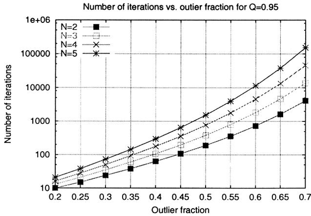
Fig. 2. Plots of the number of iterations  $m$  corresponding to different values of  $N$  and  $e$ . The probability  $Q$  is equal to 0.95 in all cases. Note the logarithmic scale in the Y-axis.
