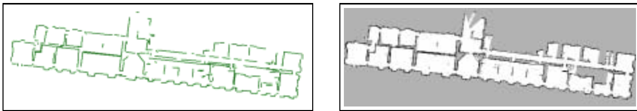
Figure 1. Line feature map (left) and occupancy grid map (right) of an exhibition site generated by the robot
