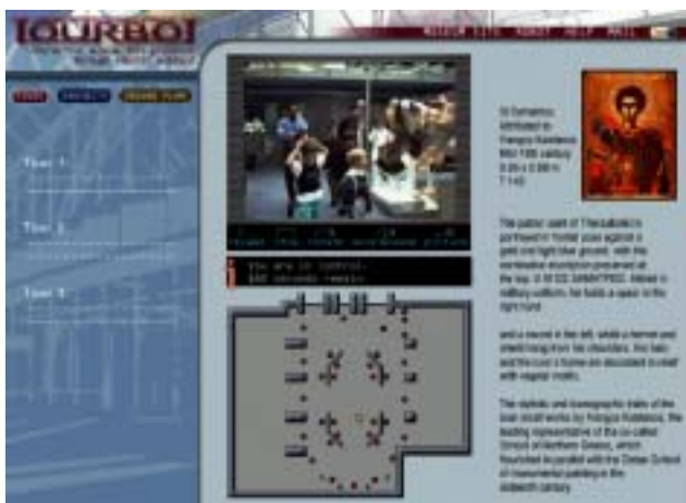
Figure 4. Web interface of the TOURBOT system for exclusive control over the robot.
