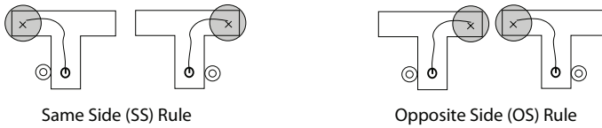
Fig. 1. A schematic representation of the response rules. The robot starts always from the bottom of the T-maze. Light cues are shown as double circles. Target locations are represented by \times , while reward corresponds to the gray area.
