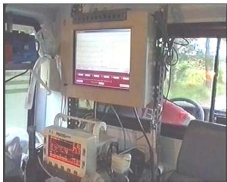
Figure 2. The internal setting of the ambulance with the panel PC and the vital sign monitoring.
