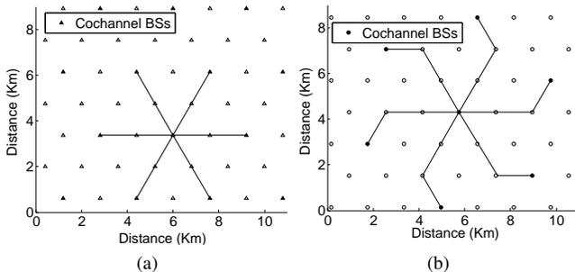
Fig. 1: Closest interfering BSs when the reuse factor is 4 (left) and 7 (right).
