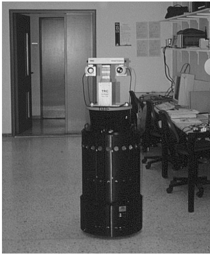
Figure 9. TALOS, the multisensor mobile robot of ICS FORTH.
