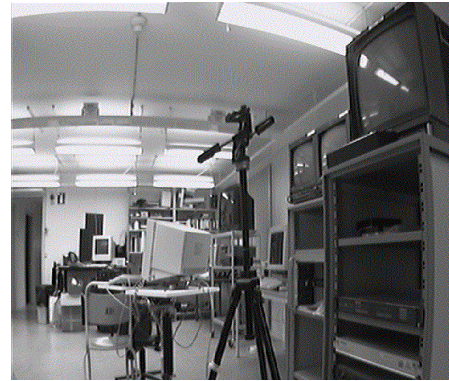
Figure 2: Example of geometric distortions produced by a wide field of view camera
