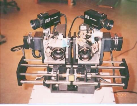
Figure 3: The KTH head with two extra cameras mounted on it for implementing peripheral vision.
