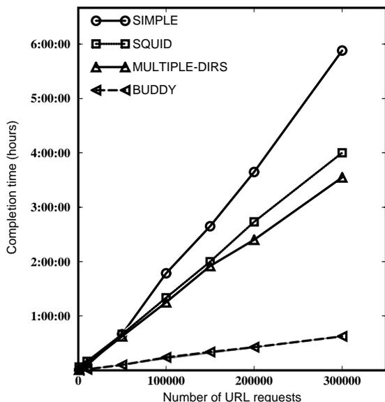
Figure 4: **File Management Overhead for Web Proxies.** The figure displays the overhead of doing 300,000 second-level cache file system operations on a 1-Gbyte disk. We see that both methods that create one file for each URL they need to store perform very bad. BUDDY, which stores several URLs per file takes roughly less than 9 msec per file operation.
