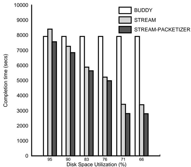
Figure 6: **Overhead of file management algorithms as a function of disk (space) utilization.** The figure displays the time it took to serve 1,000,000 file system operations as a function of disk utilization. The performance of STREAM and STREAM-PACKETIZER improves as disk utilization decreases. When disk utilization is around 70% both STREAM and STREAM-PACKETIZER outperform BUDDY by 2-3 times.
