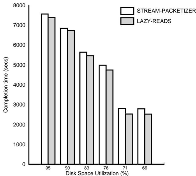
Figure 7: **Performance of LAZY-READS.** The figure displays the cost of serving 1,000,000 file system operations as a function of 2-Gbyte disk utilization. LAZY-READS gathers reads requests ten-at-a-time and issues them all at the same time to the disk reducing the disk head movements between the write stream and the data read. The figure shows that LAZY-READS improves the performance of STREAM-PACKETIZER by 10%.
