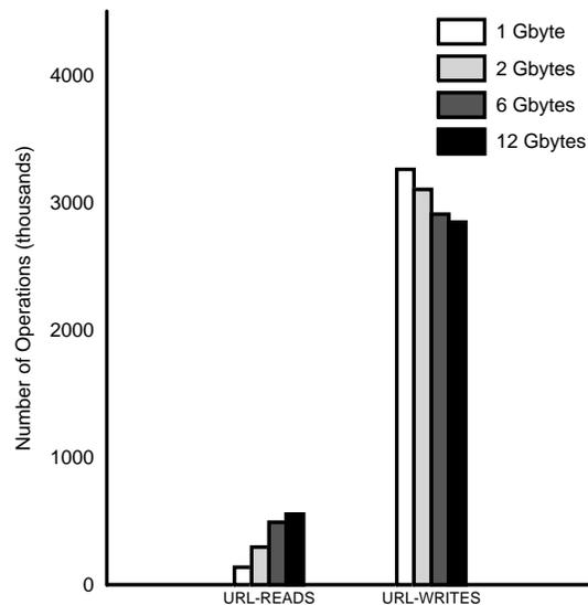
Figure 2: **File System Operations.** The figure displays the amount of URL operations (read/write) during the execution of a web proxy for various disk sizes. In all cases, write operations outnumber read operations.
