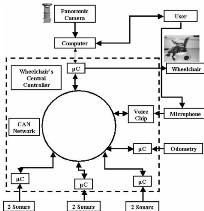
Figure 8. Hardware architecture of the robotic wheelchair.
