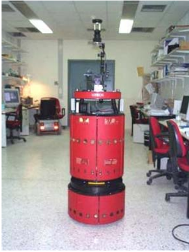
Figure 10. LEFKOS, the mobile robotic platform of ICS/FORTH with a panoramic camera mounted on it.
