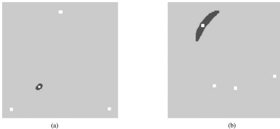
Figure 11. Influence of the arrangement of features on the accuracy of reaching a desired position. Dark gray area represents the uncertainty in position due to the error in feature localization (a) for a panoramic camera and (b) for a 60^\circ f.o.v. conventional camera.
