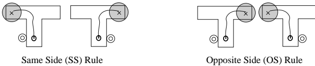
Fig. 2. A schematic representation of the delayed response rules. Light samples are represented by double circles. Goal locations are represented by \times , while reward corresponds to the gray area. The behavioral task asks for controllers capable of switching between the two rules.
