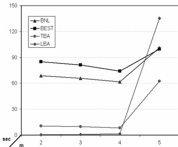
Figure 41: Total time, uniform testbed (100 MB)
