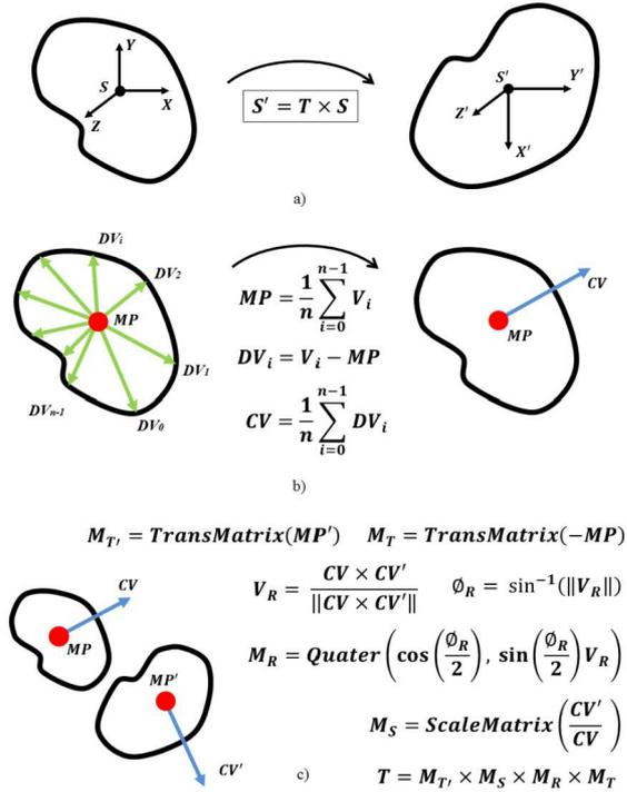
**Figure 4:** Algorithm for the geometric propagation of an Area; a) transformation between two abstract shapes with different orientation and scale, b) calculation of the characteristic vector of a shape, and c) computation of the transformation matrix
