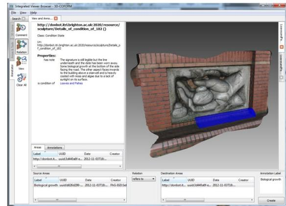
**Figure 7:** Example of area definition in the 3D shape and its enrichment with condition assessment information
