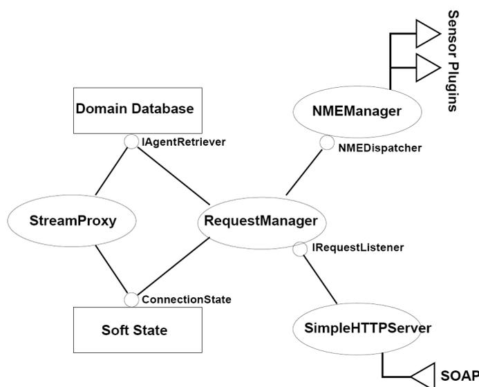
Figure 3. Modular view of a Network Monitoring Agent
