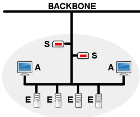
Figure 1. Deployment of *gd2* components in a Domain: E units represent generic monitoring endpoints, A labelled units represent Network Monitoring Agents, S units represent Network Monitoring Sensors
