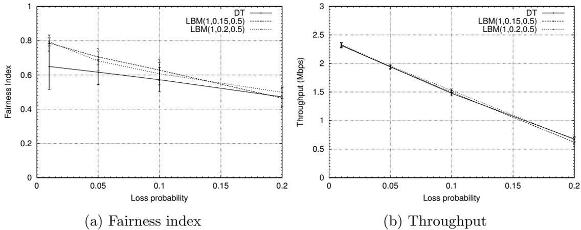
Figure 6: Fairness index and throughput for different wireless loss probabilities. LBM parameters:  $\alpha = 1$ ,  $\rho_0 = 0.15, 0.2$ ,  $t_{avg} = 500$  ms. Average file size = 500 KBytes, RTT = 20 ms, 20 FTP flows.
