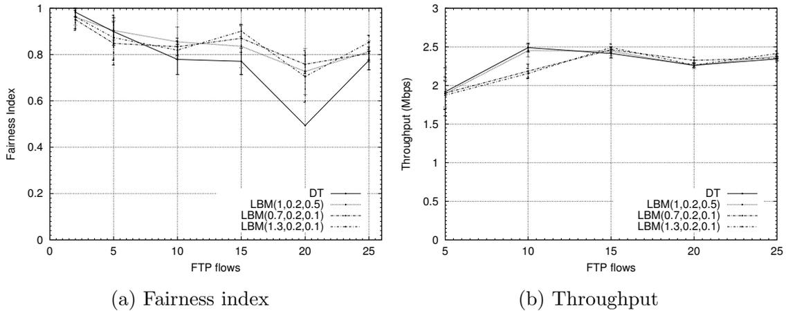
Figure 4: Fairness and throughput for different number of FTP flows. LBM parameters:  $\alpha = 1, 0.7, 1.3$ ,  $\rho_0 = 0.2$ ,  $t_{avg} = 500$  ms, 100 ms. Average file size = 500 KBytes, RTT = 50 ms, wireless loss probability = 0.01.
