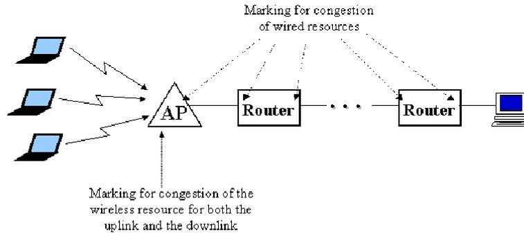
Figure 1: Routers are responsible for marking based on the congestion level at each of their wired links. On the other hand, the access point (AP) is responsible for marking based on the congestion level of the wireless resource (spectrum).
