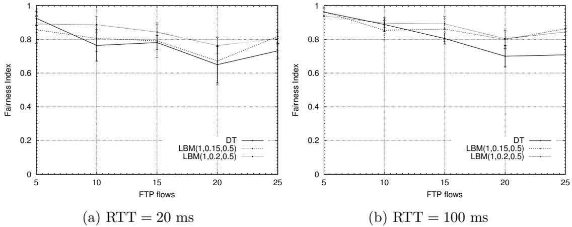
Figure 5: Fairness index for different RTT values. LBM parameters:  $\alpha = 1$ ,  $\rho_0 = 0.15, 0.2$ ,  $t_{avg} = 500$  ms. Average file size = 500 KBytes, wireless loss probability = 0.01.
