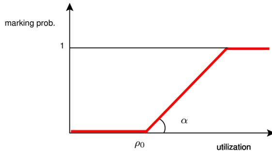
Figure 2: With load-based marking (LBM), the marking probability is a piecewise linear function of the average utilization. The LBM algorithm has three parameters: the time interval  $t_{avg}$  over which the aggregate utilization is measured, the minimum utilization  $\rho_0$ , and the slope parameter  $\alpha$ .
