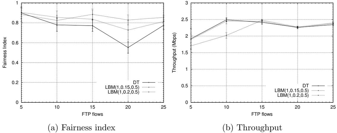
Figure 3: Fairness and throughput for different number of FTP flows. LBM parameters:  $\alpha = 1$ ,  $\rho_0 = 0.15, 0.2$ ,  $t_{avg} = 500$  ms. Average file size = 500 KBytes, RTT = 50 ms, wireless loss probability = 0.01.
